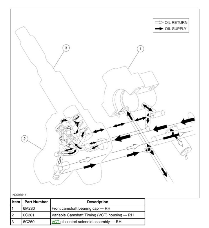
Variable Camshaft Timing (VCT) Housing
